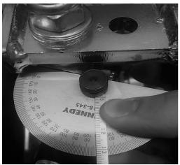
Rotate clevis mount 17 degrees clockwise.
