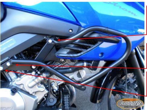
bolt M8x50mm to frame gripping+ duralumin cylinder 16mm + pad (spring) + cover on head of bolt
