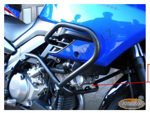
bolt M8x30mm to connect left and right side
