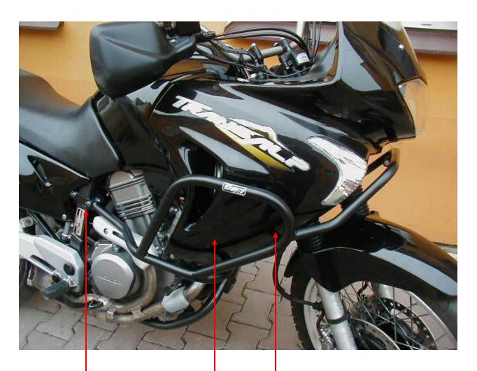
two bolts M8x50mm + two pads (spring) + two coves on head of bolts + steel adapter for connecting of the left and right crash bar with frame of the motorcycle; bolt M8x110mm + two pads (plane) + nut M8 (safety)
