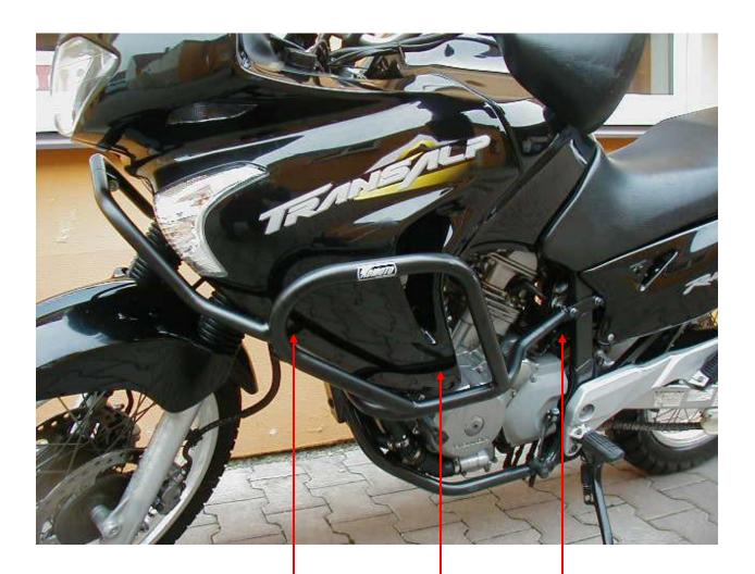
for connecting of the crash bar with frame of the motorcycle; bolt M6x30mm + pad (plane) for connecting of the left and right crash bar with frame of the motorcycle (viz the right side)
