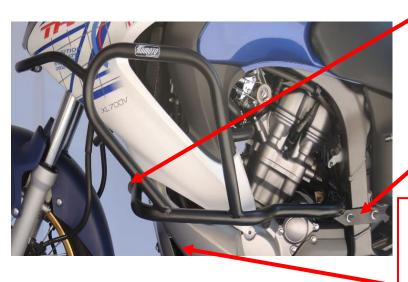
Frame fixed on the steel adapter with screw M10 (note 9) and spring washer.
