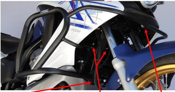
On the frame instalation of steel adapter (not. 1), stick on it 3M sticker (not.12). Steel adapter mount with stainless bracket (not. 2). For fixed use washers and nuts (not. 3.,4.) Put the plastic cover (note 5.)
