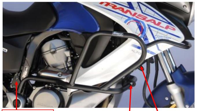
Note 2. Aluminium cylinder D 27 put between crash frame and bike frame Fixed with screws and washers (note. 3.,4.) Plast. cover
