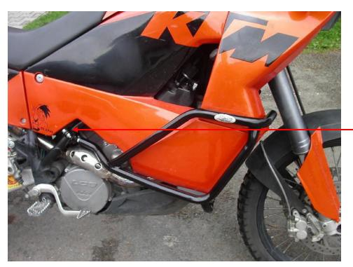
steel adapter with thread M10 + steel adapter on bar  $\emptyset$  = 25mm + two bolts M8x25mm + four pads M8 (plane) + two nuts M8 (safety)
