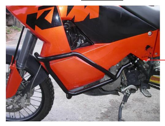
steel adapter with thread M10 + steel adapter on bar  $\emptyset$  = 25mm + two bolts M8x25mm + four pads M8 (plane) + two nuts M8 (safety)
