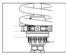
Rebound damping:-Bottom Adjuster Wheel:- 32 clicks adjustment range. All settings should be made from the fully closed (Clockwise Position).
