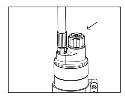
Compression damping:-Black Adjuster Knob:- 30 clicks adjustment range. All settings should be made from the fully closed (Clockwise Position).
