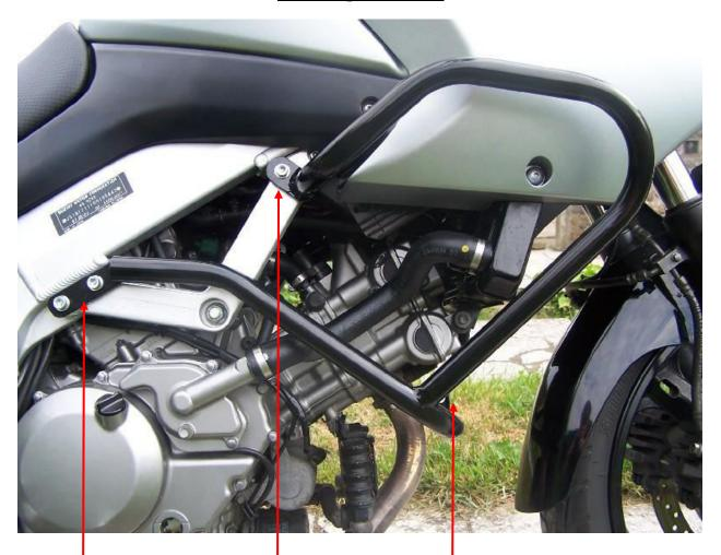
two bolts M8x50mm + two duralumin cylinders 13mm + two pads (spring) + two covers on head of bolt bolt M8x50 mm + cylinder 13mm + pad (spring) + cover on head of bolt for connecting of the left and right side of the crash bars; bolt M8x30mm
