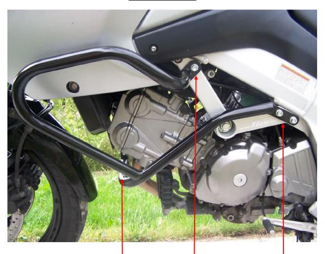
for connecting of the left and right side of the crash bars (viz the right side) bolt M8x50 mm + cylinder 13mm + pad (spring) + cover on head of bolt two bolts M8x50mm + two duralumin cylinders 13mm + two pads (spring) + two covers on head of bolt
